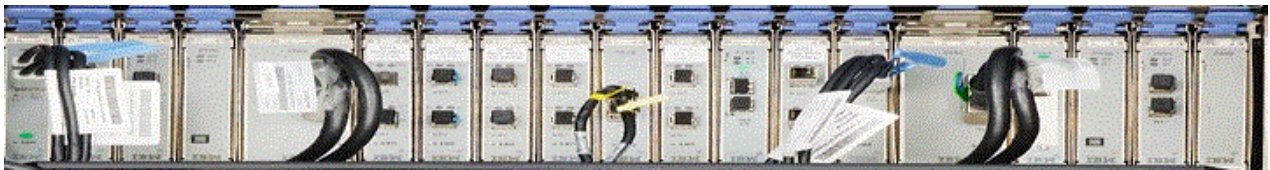
Figure 46. Photograph of a physical adapter card in a system I/O drawer
